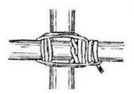
Finish off the lashing with a clove hitch around the cross member. Dress the knot and keep it tight.
