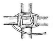
Then you change the direction of the wraps or "fraps" by circling around the first set of wraps 2 to 3 times to further tighten and secure the lashing.
