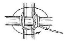
This pattern is repeated until you form 3 to 4 tight wraps around each of the staffs or spars forming the lash. Be sure to tighten each wrap along the way.
