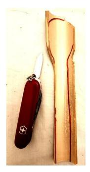
Layout your spoon shape and draw it on the interior of the curved section of bamboo. Ensure that you allow at least 1/2 of an inch at the top edge of the scoop end to allow the carving of a symmetric tip. Begin to carve out your spoon making long paring cuts to the handle sides, starting from the scoop end and cutting toward the end of the handle. Make small trimming cuts to round the top of the scoop. The small blade is best for these carving tasks.
