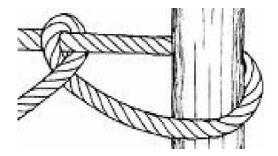
Wrap the cordage around the post or staff, and pass the working end of the cordage thru the opening.
