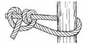
Wrap the cordage around the main strand of the cordage and pass the end of the cordage thru the eye ensuring that the end exits in opposition to the entry of the first loop. Tighten and dress the knot.
