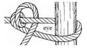
Pass the end of the cordage thru the eye a second time forming a double wrap thru the loop.
