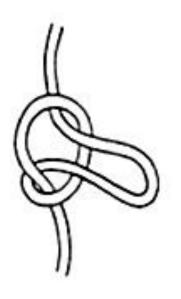
Grab the standing end of the cordage and pull a small bight thru the center of the eyelet.
