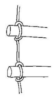
Used in a series, the marlinspike hitch can be used to fashion a ladder with simple timbers cut to length and inserted at even intervals along the rope.
