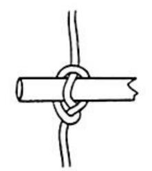
Insert the marlinspike (or other implement), and tighten the knot by pulling the standing end of the cordage and dressing the knot.
