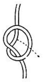
Then slide the eyelet over the front of the standing end of the cordage covering the standing end, and allowing for the standing segment of cordage to be passed forward thru the eyelet.
