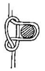
The downward tension on the knot keeps the lower loop of the knot fixed and prevents slipping; once the tension is released, the marlinspike (or other implement) can easily be removed, and the knot will simply slip out.
