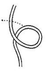
Start by forming an eyelet from the standing end (long end) of the cordage by bringing the running end (shorter end) under the standing end.
